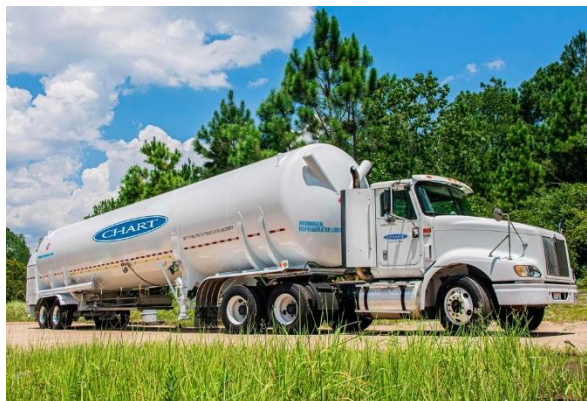
Figure 10. A large-scale liquid hydrogen truck [26]
